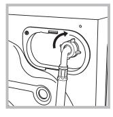
1. Connect the inlet hose to the machine by screwing it onto the cold water inlet of the appliance, which is situated on the top righthand side of the rear part of the appliance (see figure).
